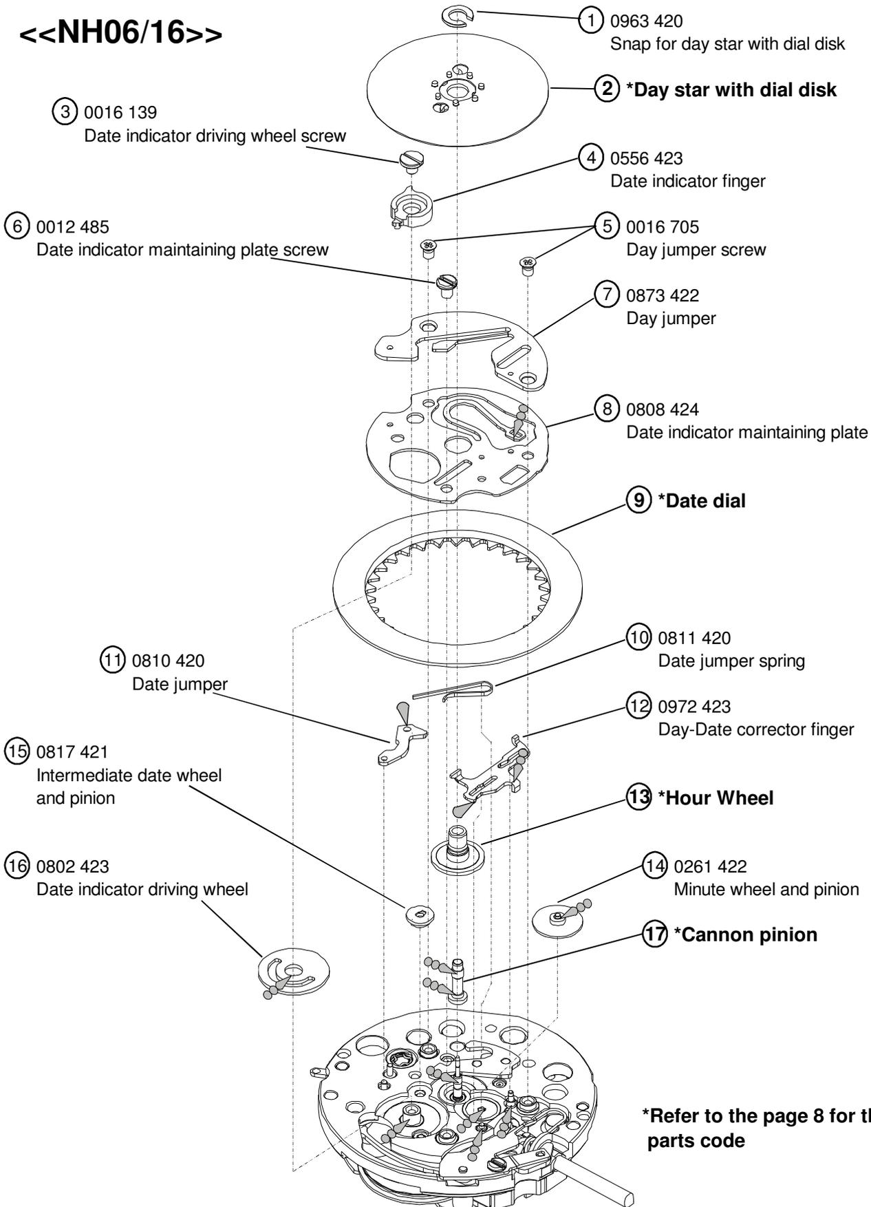
Disassembling procedures Figs. ① → ④⑩
